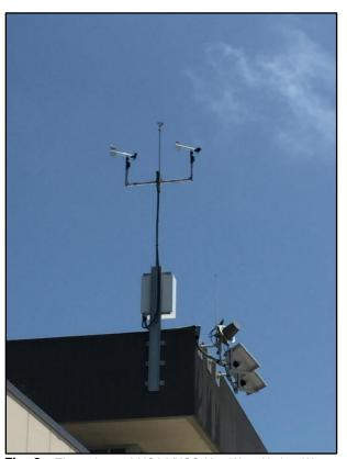
**Fig. 2.** The re-located NOAA/NOS Key West Harbor Water Level Observation Network anemometers, atop the NOAA/FKNMS administration building, Key West, Florida.
